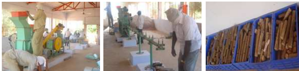
Figure 2. Processing of briquette into final product briquettes
