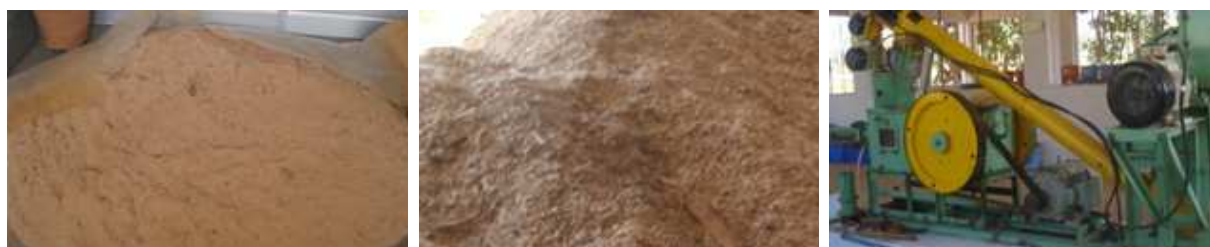
Figure 1. Raw material used to prepare briquettes and briquetting machine
