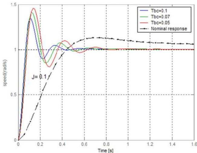
FIGURE 7. System Test Results with PID Controller
