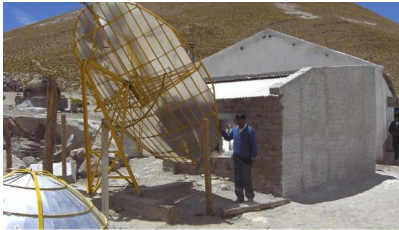
Figure 5: Solar community oven powered by Scheffler reflector
