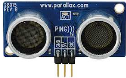
Gambar 6. Sensor Ultrasonic PING))) Parallax (sumber: (Mc Comb, 2012))
