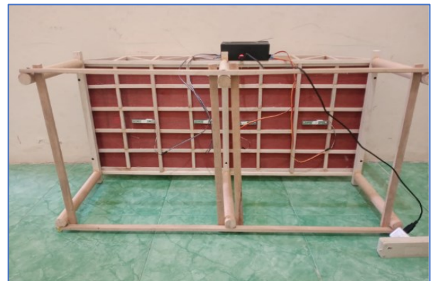
FIGURE 7. Installing the Detector on a Miniature Bridge
