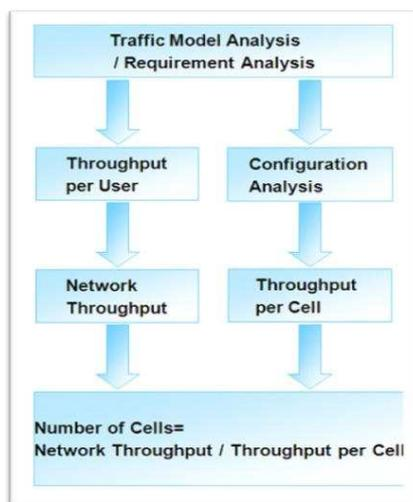
Gambar 14. Diagram Alur LTE Capacity Dimensioning (Huawei, 2010)
