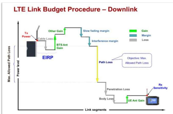
Gambar 13. Link Budget Arah Downlink (Huawei Technologies co.,LTD, 2010)
