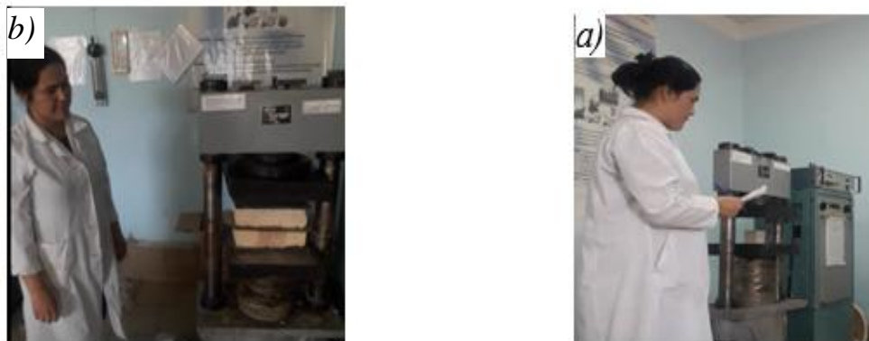
Figure 2: Test of brick compression (a) and mortar (b)
