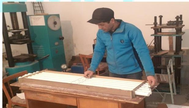
Fig.4. Hollow core formwork
