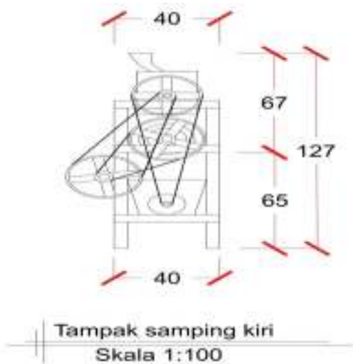
Gambar 2. Tampak Samping kanan Re-desain Alat Perontok Bunga Cengkeh
