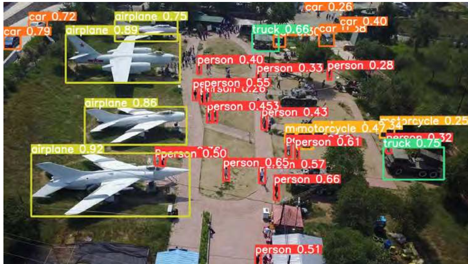
Fig. 6. Object detection in an aerial photograph from the VisDrone set in Colab Notebooks using the YOLOv5x model
