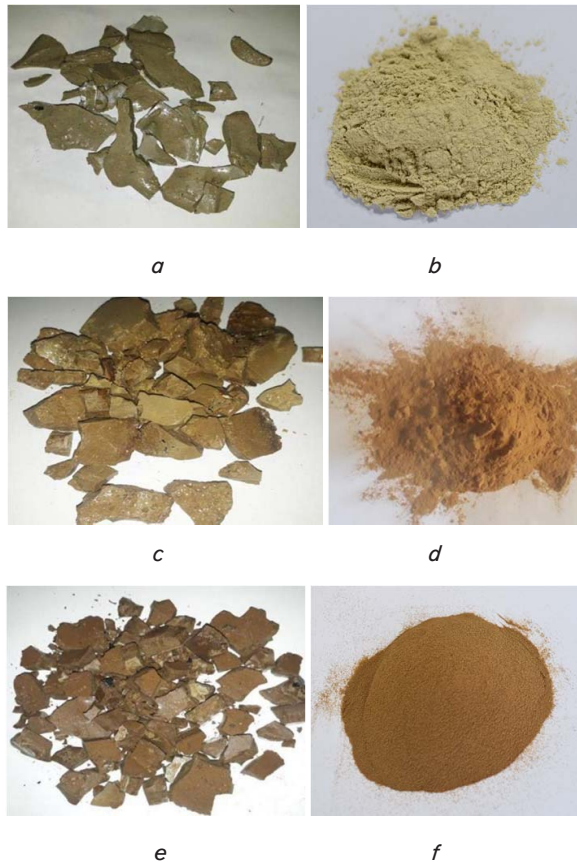
Fig. 2. The form of a melt of recycled waste after cooling and RCCF 75 µm at different heating time: a, b – 2 min; c, d – 4 min; e, f – 6 min
