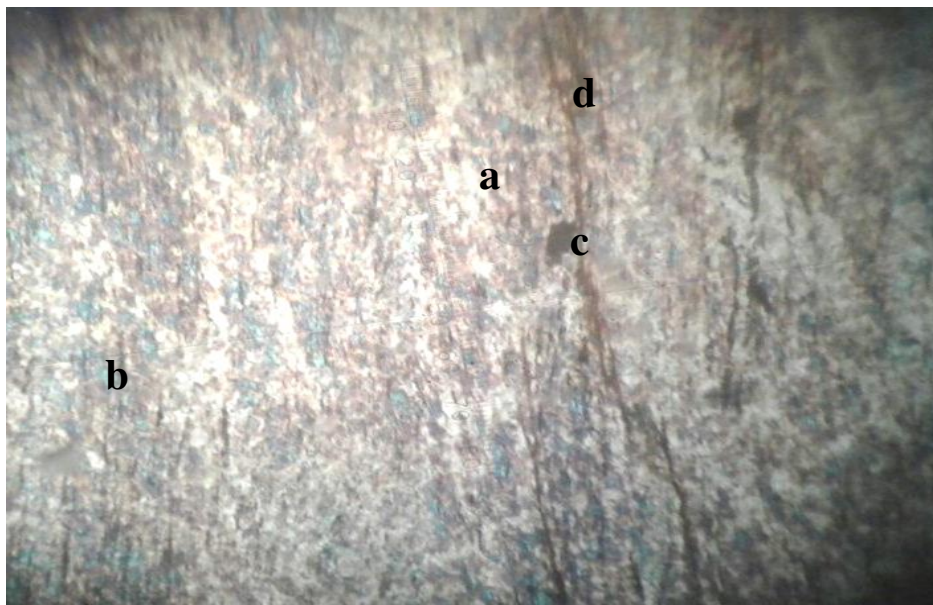
Figure 9. Schist chlorite rock in the small slice: (a) muscovite, (b) chlorite, (c) opaque mineral, (d) oxide mineral
