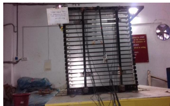
Figure 3. Laminar box mounted on shake table
