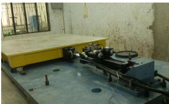
Figure 2. Shake table test apparatus
