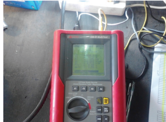
Gambar 9. Alat Ukur Power Quality DM III Multitest
