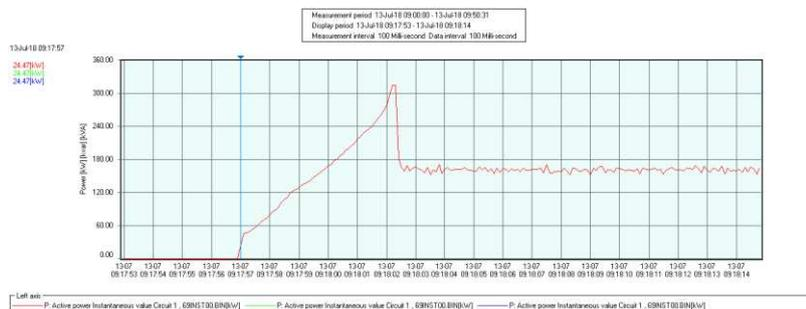
**Gambar 7. (c)** Tampilan grafik hasil pengukuran daya motor pompa PA – 03 AP001
