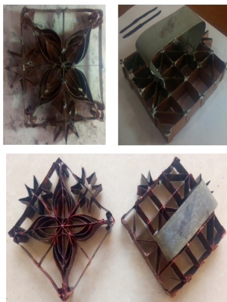
Figure 7. Third test using Harris's patri (upper picture set shown the motif and handle before soldering process; bottom picture shown the motif and handle after soldering process)
