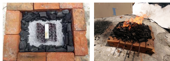
Figure 1. Conventional soldering process of stamp batik
