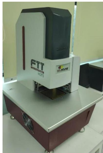
**Gambar 1.** Fabric Touch Tester (FTT)
