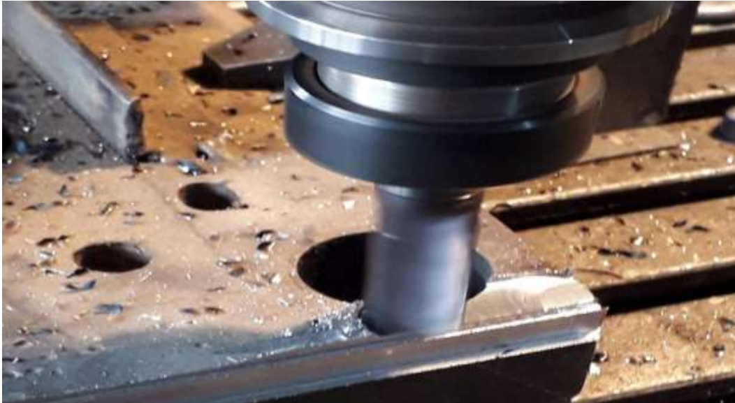
Figure 4. The process of processing with the help of finger milling
