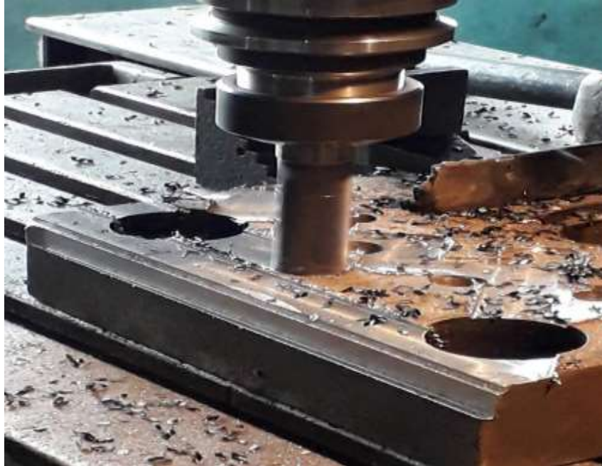
Figure 3: Detail separation process during machining.
