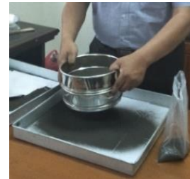
Figure 12. Iron Sand Sample Screening Process
