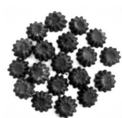
Gambar 13. Pellet Besi Hasil Proses Microwave
