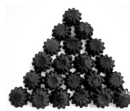
Gambar 14. Pellet Besi Campuran Silika Hasil Proses Microwave
