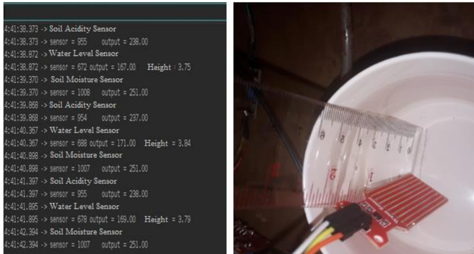
(a) Water level sensor testing via serial monitor (b) Measurement using a ruler
