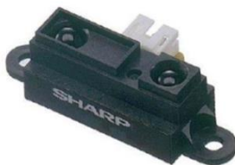
Gambar 2. Sensor Sharp 2Y0A21 (Sumber : www.saptaji.com , 2020)
