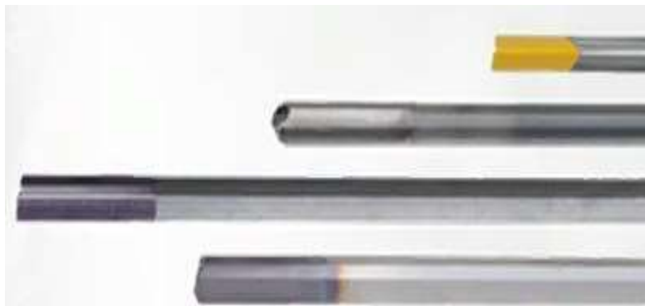
Fig. 1. Gun drills with coatings deposited
