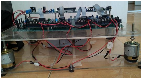
Figure 3. Simulation table of cannon position using accelero sensor
