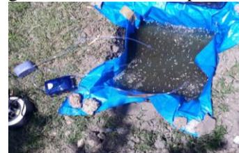
**Gambar -9 :** *Oxidation Pond* Skala Laboratorium
