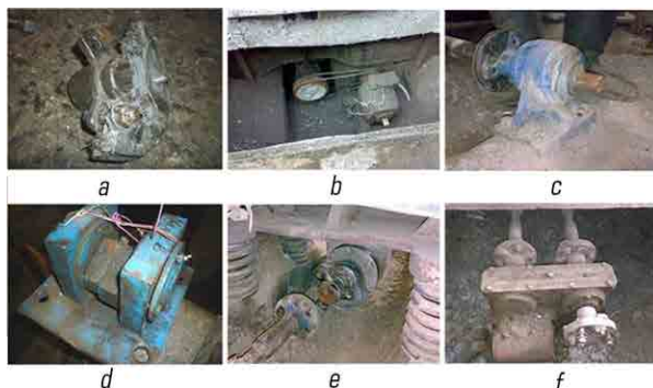
Fig. 7.17 Photo fixation of failures of mechanical assemblies and parts of vibration platforms: a – failure of the coupling; b – failure of the electric motor; c – failure of the bearing assembly; d – failure of the vibration block; e – failure of the propeller shaft; f – failure of the synchronizer
