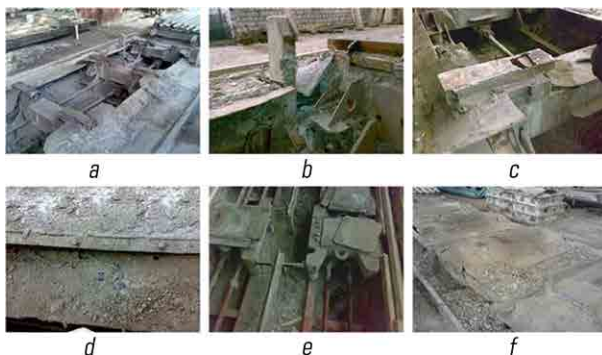
Fig. 7.18 Photo fixation of failures of the working bodies of vibration platforms: a – failure of vibration plates; b – deformation of the limiters; c – damage to the contact platform; d – damage to the protective casing; e – damage to vibration plates; f – blockage of the vibration platform
