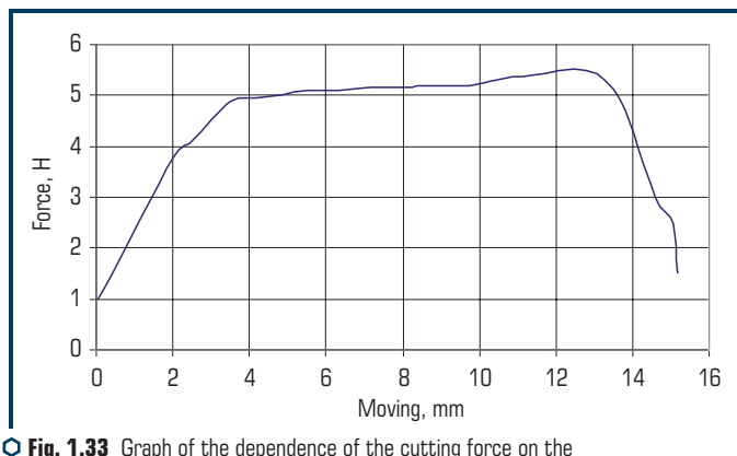
Fig. 1.33 Graph of the dependence of the cutting force on the movement of the knife when cutting the pulp of Ternek melon variety
