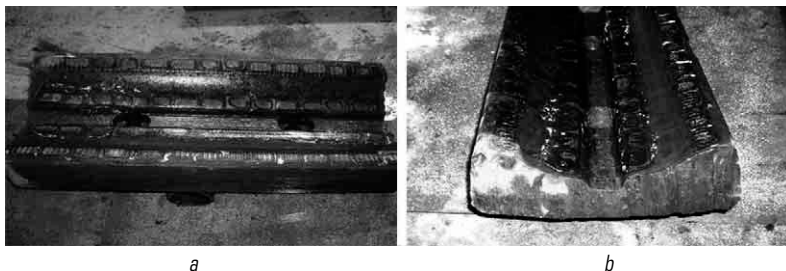
○ Fig. 2.63 Lining of a heavy ball mill after hardening: a – top view; b – view from the lining end
