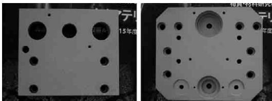
○ Fig. 5.18 Parts of die tooling with ceramic coating
