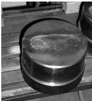
○ Fig. 10.4 Hardened die for hot forming of cleaning machine cutters
