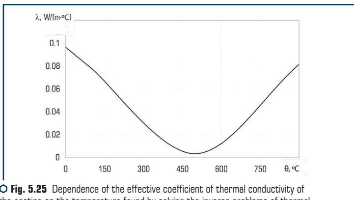
**Fig. 5.25** Dependence of the effective coefficient of thermal conductivity of the coating on the temperature found by solving the inverse problems of thermal conductivity, according to the indicators of three thermocouples
