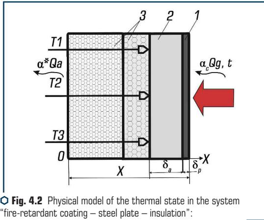
**Fig. 4.2** Physical model of the thermal state in the system "fire-retardant coating – steel plate – insulation":
