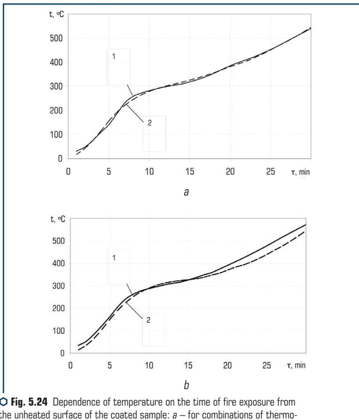
**Fig. 5.24** Dependence of temperature on the time of fire exposure from the unheated surface of the coated sample: *a* – for combinations of thermocouples T2–T3 and T1–T3; *b* – for combinations of thermocouples T2–T1; 1 – experimental curve; 2 – calculated curve
