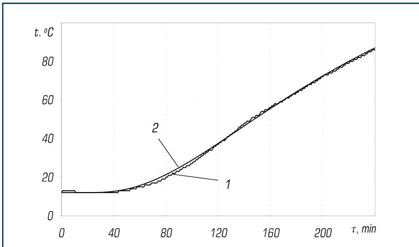
**Fig. 3.10** Dependence of temperature on time of fire influence from unheated surface of fire-protected reinforced concrete floor: 1 – experimental temperature from unheated surface; 2 – design temperature obtained by solving the inverse problems of thermal conductivity
