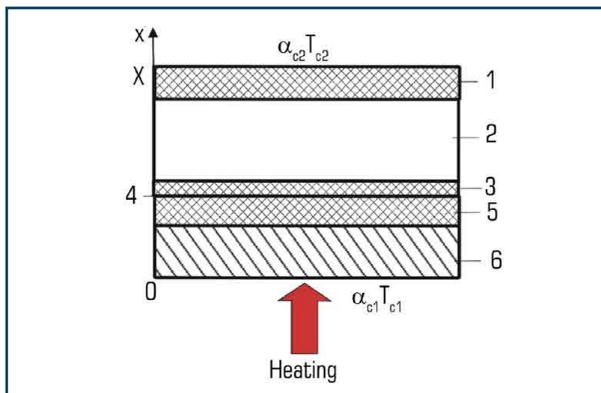
○ **Fig. 5.4** Scheme of multi-hollow reinforced concrete floor in one-dimensional formulation: 1 – a layer of solid concrete between the unheated surface and the layer with floor cavities; 2 – layer with voids; 3 – a layer of solid concrete between the cavities and reinforcement; 4 – armature layer; 5 – a layer of solid concrete from the reinforcement to the heated surface; 6 – plaster coating
