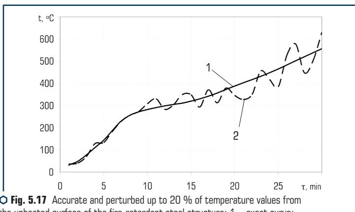
○ **Fig. 5.17** Accurate and perturbed up to 20 % of temperature values from the unheated surface of the fire-retardant steel structure: 1 – exact curve; 2 – perturbed by 20 % curve
