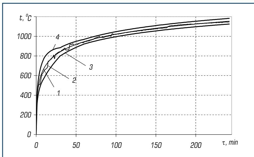
**Fig. 3.6** Dependence of the temperature in the furnace on the time of fire exposure on the heating surface of the fire-retardant reinforced concrete multi-hollow slab with a thickness of 220 mm: 1 – curve of standard temperature regime; 2 – real curve of temperature change in the furnace; 3 – the minimum values of temperature in the furnace are admissible at tests; 4 – the maximum values of temperature in the furnace are admissible at tests
