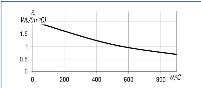
○ **Fig. 3.8** Dependence of the effective coefficient of thermal conductivity of concrete of fire-retardant reinforced concrete multi-hollow floor on temperature, obtained as a result of solving the inverse problems of thermal conductivity according to fire resistance tests
