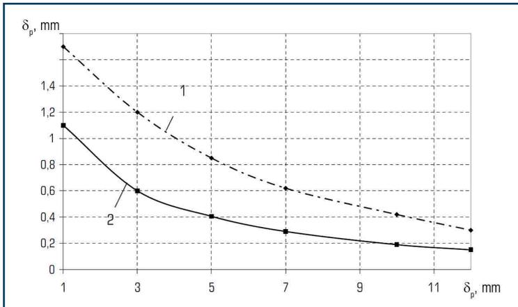
**Fig. 4.21** Dependence of the minimum thickness of the investigated fire-retardant coating ( $\delta_p$ ) on the thickness of the steel plate ( $\delta$ ) for the critical steel temperature of 500 °C and the normalized duration of fire exposure of 30 minutes: 1 – at the temperature of hydrocarbon fire; 2 – at standard fire temperature
