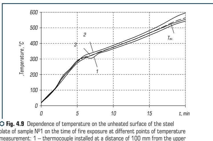
**Fig. 4.9** Dependence of temperature on the unheated surface of the steel plate of sample N°1 on the time of fire exposure at different points of temperature measurement: 1 – thermocouple installed at a distance of 100 mm from the upper edge of the plate; 2 – thermocouple mounted in the center of the plate; 3 – thermocouple installed at a distance of 100 mm from the lower edge of the plate;  $T_{av}$  – the average value of the three thermocouples
