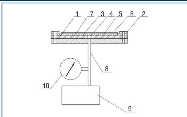
**Fig. 5.32** Scheme of the installation to determine the adhesive strength of the coating: 1 – plate; 2 – frame; 3 – substrate; 4 – hole; 5 – coverage; 6 – safety cover; 7 – seals; 8 – fitting; 9 – compressed gas supply mechanism; 10 – manometer
