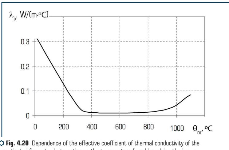
**Fig. 4.20** Dependence of the effective coefficient of thermal conductivity of the investigated fire-retardant coating on the temperature found by solving the inverse problems of thermal conductivity
