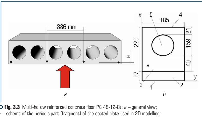
**Fig. 3.3** Multi-hollow reinforced concrete floor PC 48-12-8t: *a* – general view; *b* – scheme of the periodic part (fragment) of the coated plate used in 2D modelling: 1 – heating surface; 2 – fire-retardant coating; 3 – reinforced concrete floor; 4 – unheated surface; 5 – cavity (round cavity) floor
