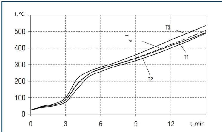
**Fig. 4.17** Dependence of temperature from the unheated surface of the steel plate on the time of fire exposure at different points of temperature measurement: T1 – thermocouple installed at a distance of 100 mm from the upper edge of the plate; T2 – thermocouple installed in the center of the plate; T3 – thermocouple installed at a distance of 100 mm from the lower edge of the plate;  $T_{av}$  – the average value of the three thermocouples
