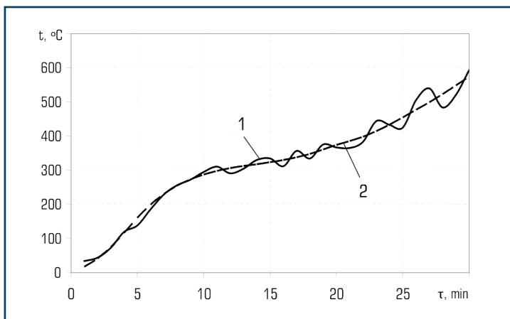
○ **Fig. 5.19** Experimental and calculated values of temperatures from the unheated surface of the fire-retardant steel structure during their perturbation by 10 %: 1 – experimental curve; 2 – calculated curve
