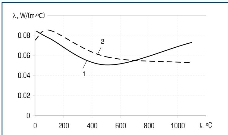
○ **Fig. 5.3** Dependence of the effective coefficient of thermal conductivity of the investigated plaster coating on temperature: 1 – exact coefficients; 2 – coefficients obtained by solving the inverse problems of thermal conductivity at perturbed temperatures by 10 %
