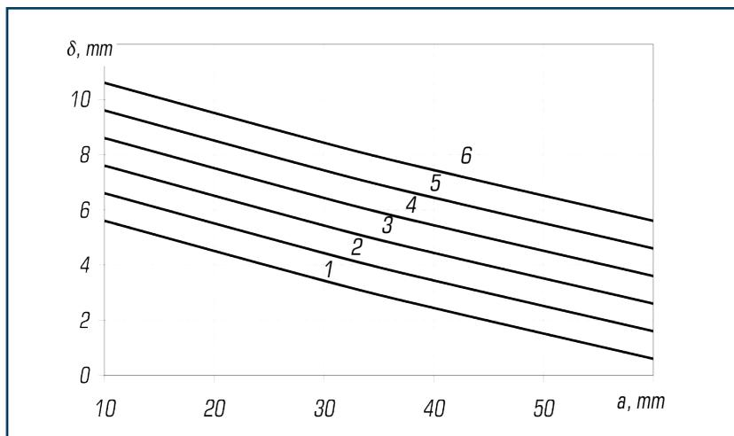
**Fig. 3.11** Dependence of the thickness ( $\delta$ ) of “Neospray” plaster coating on the thickness of the protective layer of concrete of multi-hollow reinforced concrete floor ( $a$ ) according to the criterion of reaching the critical temperature of reinforcement ( $500\text{ }^{\circ}\text{C}$ ) for fire resistance: 1 – 60 minutes; 2 – 90 minutes; 3 – 120 minutes; 4 – 150 minutes; 5 – 180 minutes; 6 – 240 minutes
