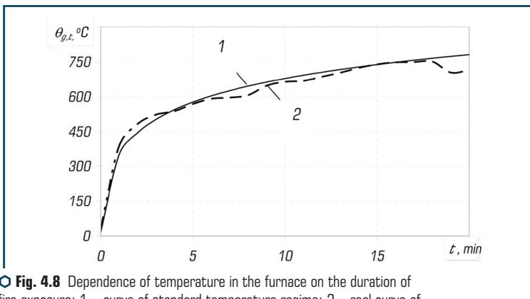
**Fig. 4.8** Dependence of temperature in the furnace on the duration of fire exposure: 1 – curve of standard temperature regime; 2 – real curve of temperature change in the furnace
