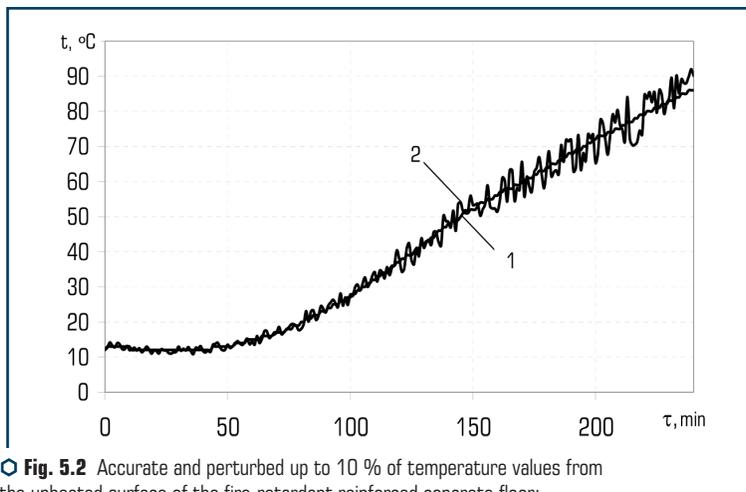
**Fig. 5.2** Accurate and perturbed up to 10 % of temperature values from the unheated surface of the fire-retardant reinforced concrete floor: 1 – exact curve; 2 – curve perturbed by 10 %
