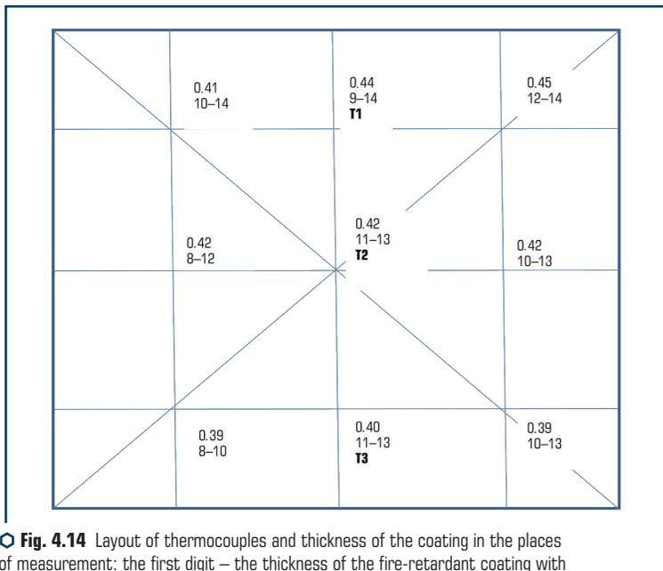
**Fig. 4.14** Layout of thermocouples and thickness of the coating in the places of measurement: the first digit – the thickness of the fire-retardant coating with soil, mm; the second digit – the thickness of the swelling, mm; the third digit – the location of the thermocouple
