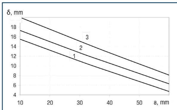
○ **Fig. 5.8** Characteristics of fire-retardant ability of the investigated plaster coating according to the criterion of reaching the critical temperature of reinforcement (500 °C) for the limit of fire resistance of 180 minutes: 1 – for standard temperature regime; 2 – for the hydrocarbon fire mode; 3 – for tunnel fire mode according to Dutch standards (RWS)
