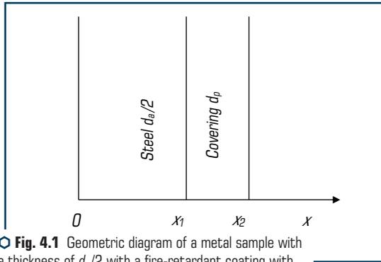
Fig. 4.1 Geometric diagram of a metal sample with a thickness of  $d_s/2$  with a fire-retardant coating with a thickness of  $d_p$
