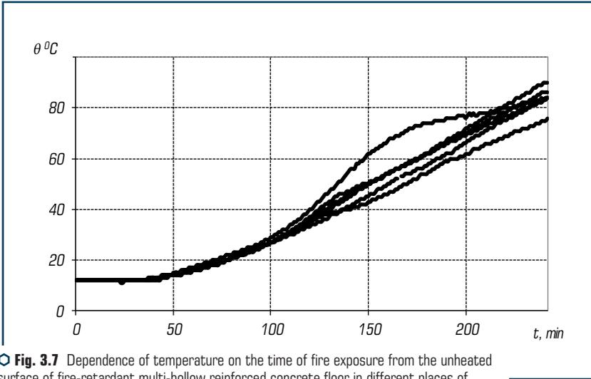
○ **Fig. 3.7** Dependence of temperature on the time of fire exposure from the unheated surface of fire-retardant multi-hollow reinforced concrete floor in different places of temperature measurement
