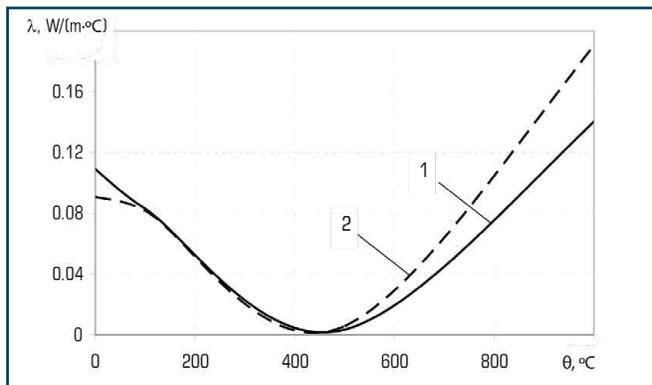
○ **Fig. 5.18** Dependence of the effective coefficient of thermal conductivity of fire-retardant coating on temperature, where: 1 – exact coefficients; 2 – coefficients obtained by solving the inverse problems of thermal conductivity at perturbed temperatures by 10 %
