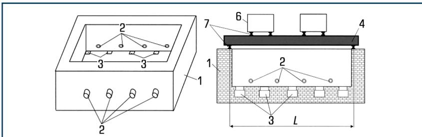
○ **Fig. 2.3** Scheme of the horizontal furnace: 1 – furnace body; 2 – burners; 3 – channels for exhaust gases; 4 – sample being tested; 5 – thermocouples in the furnace; 6 – load on the sample; 7 – hinged supports
