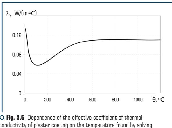
Fig. 5.6 Dependence of the effective coefficient of thermal conductivity of plaster coating on the temperature found by solving the inverse problems of thermal conductivity according to fire resistance tests
