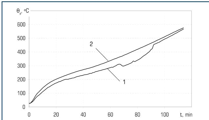
○ **Fig. 5.12** Dependence of average temperatures of samples of steel columns with fire-retardant coating “Amotherm Steel Wb” on the time of fire exposure to the standard temperature of the fire: 1 – sample column № 1; 2 – sample column № 2
