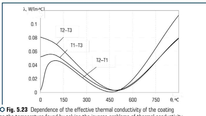
**Fig. 5.23** Dependence of the effective thermal conductivity of the coating on the temperature found by solving the inverse problems of thermal conductivity on the indicators of two thermocouples in different combinations
