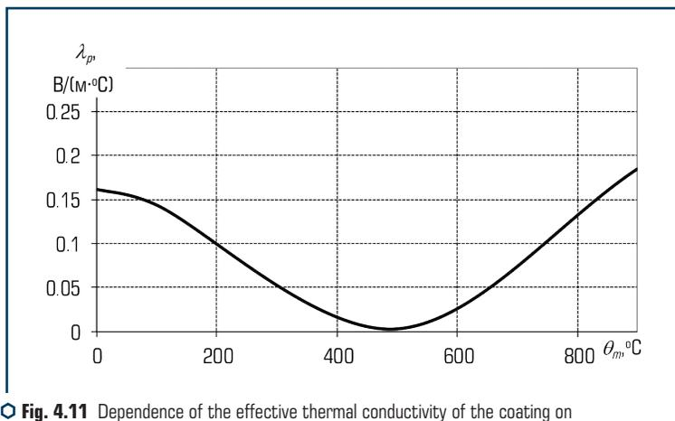
**Fig. 4.11** Dependence of the effective thermal conductivity of the coating on temperature, found by solving the inverse problem of thermal conductivity
