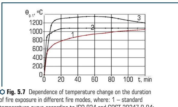
Fig. 5.7 Dependence of temperature change on the duration of fire exposure in different fire modes, where: 1 – standard temperature curve according to ISO 834 and GOST 30247.0-94; 2 – hydrocarbon curve according to EN 1363-2:1999; 3 – tunnel curve according to Netherland's standards (RWS)
