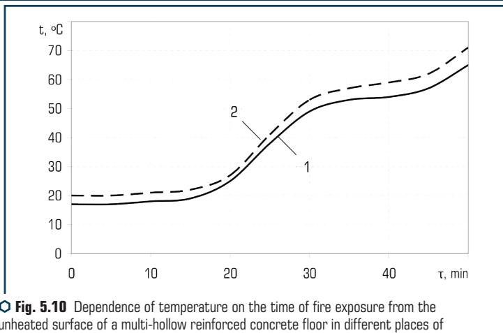
**Fig. 5.10** Dependence of temperature on the time of fire exposure from the unheated surface of a multi-hollow reinforced concrete floor in different places of temperature measurement: 1 – temperatures found during the fire resistance test; 2 – when modelling in the software package ANSYS R17.1
