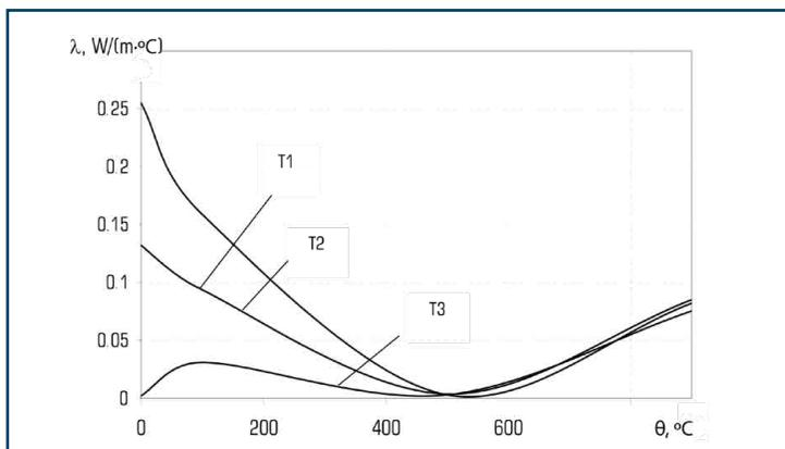
**Fig. 5.22** Dependence of the effective coefficient of thermal conductivity of the investigated coating on the temperature found by solving the inverse problems of thermal conductivity: T1 – by thermocouple located at a distance of 100 mm from the upper edge of the fire-retardant plate; T2 – according to the thermocouple located in the center of the fireproof plate; T3 – according to the thermocouple located at a distance of 100 mm from the lower edge of the flame retardant plate
