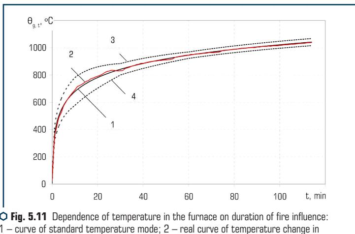
**Fig. 5.11** Dependence of temperature in the furnace on duration of fire influence: 1 – curve of standard temperature mode; 2 – real curve of temperature change in the furnace; 3 – the maximum values of temperature in the furnace are admissible at tests; 4 – the minimum values of temperature in the furnace are admissible at tests
