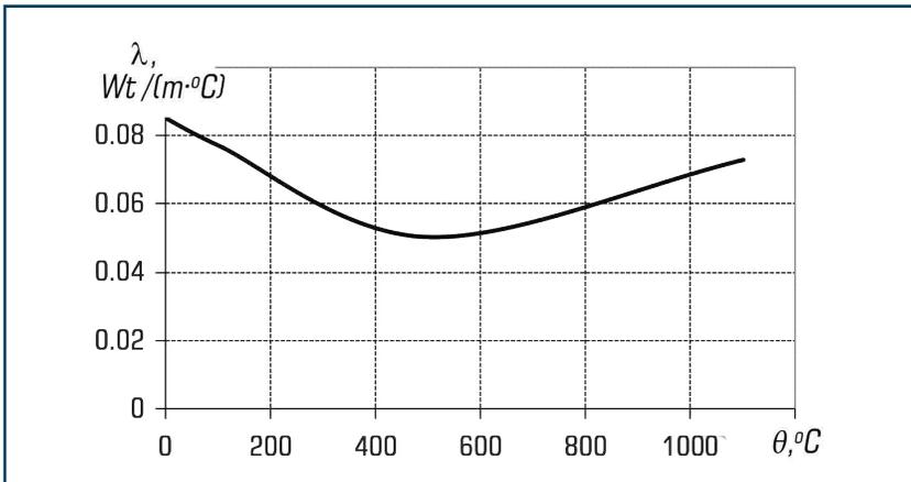
○ **Fig. 3.9** Dependence of the effective coefficient of thermal conductivity of plaster coating on the temperature found by solving the inverse problems of thermal conductivity according to the tests of fire resistance of fire-resistant multi-hollow reinforced concrete floor
