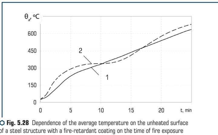
**Fig. 5.28** Dependence of the average temperature on the unheated surface of a steel structure with a fire-retardant coating on the time of fire exposure according to the standard temperature of the fire (minimum value of the coating thickness): 1 – obtained experimentally; 2 – obtained by simulation in ANSYS
