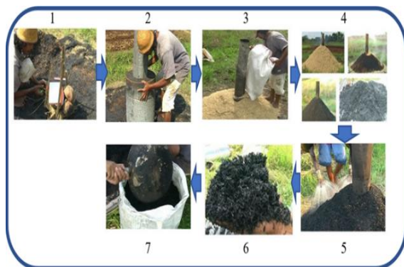
Figure 1. Production Process of Making Rice Husk Charcoal
