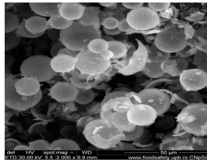
(d)<sub>1</sub> SEM of HGB<sub>sca</sub> at 2 000x
