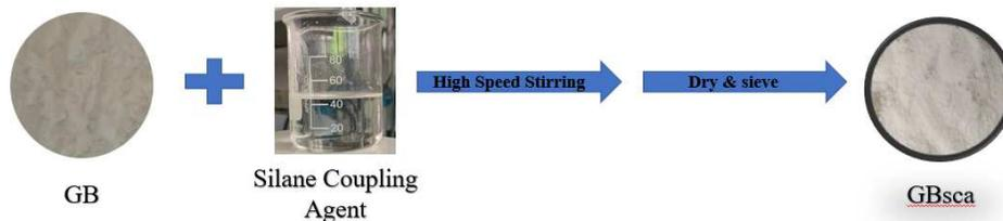
*Figure 3: Schematic illustration of preparing procedure for the Glass Bubbles and Silane Coupling Agent*
