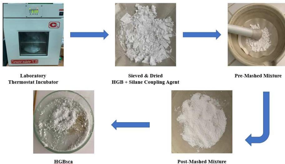
Figure 5: Schematic illustration of drying and mashing the treated Hollow Glass Bubbles<sup>3</sup>
