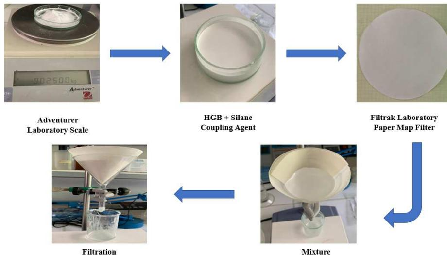
*Figure 4: Schematic illustration of preparation, mixture and filtration for the Glass Bubbles and Silane Coupling Agent<sup>3</sup>*
