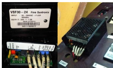
Gambar 3. Fine suntronix VSF30-24 power supply 24V 1,5A
