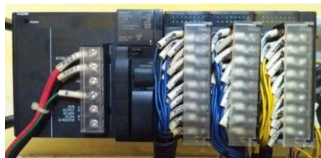
Gambar 2. PLC Omron CJ2M CPU11
