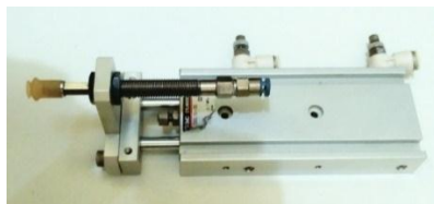
Gambar 13. Dual-rod cylinder SMC pneumatik guided cylinder CXSL10-50-XB9
