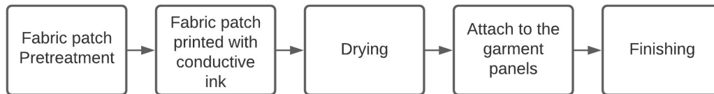
Fig. 2: Application of digital printing to produce of fabric patch for e-textiles
