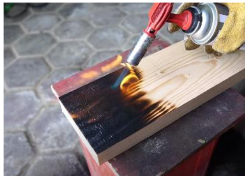
Figure 2. Burn Process with a Blowtorch [Source : Youtube Video [6]]
