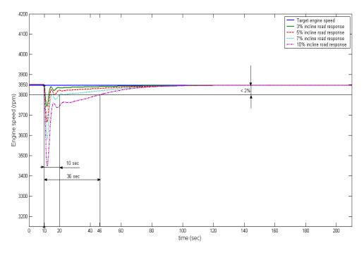
Figure 4. Performance of adaptive ANN controller for constant throttle and various road gradients
