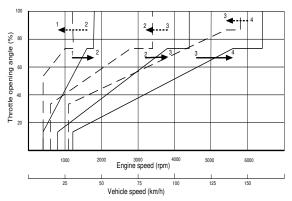
Figure 1. A typical automatic transmission shift pattern
