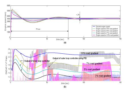
Figure 3. Performance of PID controller as outer loop controller at 80% throttle opening with road gradient variation
