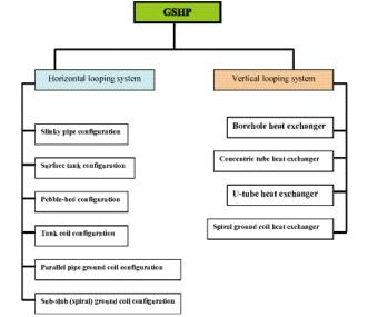
Figure 7. Common types of ground-loop heat exchangers [7]
