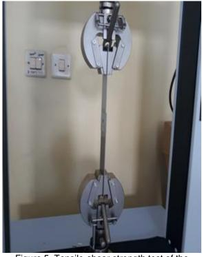
Figure 5. Tensile-shear strength test of the coupon on UTM
