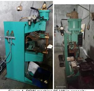
Figure 4. RSW machine 35 kW in capacity
