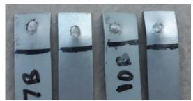
Figure 7. Interfacial Failure Mode
