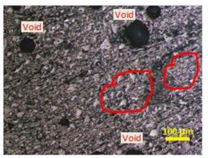
Figure 6. Cross-sectional morphology of polymerbasalt composite with a variation of 270 mesh-75% basalt powder-1/20 catalyst
