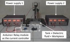
Figure 11. Proposed EDM setup
