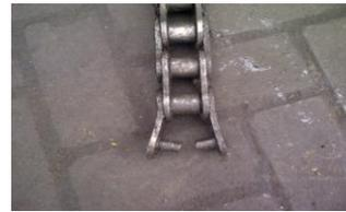
Gambar Pin Rantai Gantry RTG Putus/ Patah
