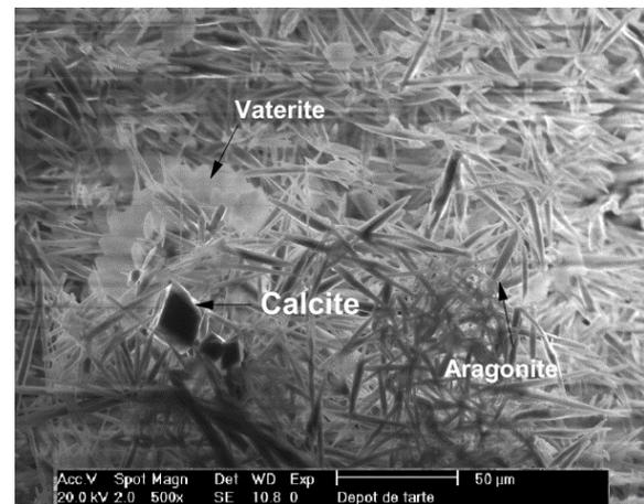
Fig 14. Surface morphology of scale deposit at -1.2 V/SCE.
