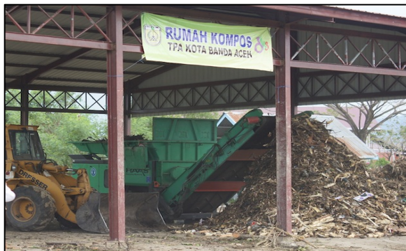
Figure 2. Mobile waste shredding machine in operation in GJL (Faisal, 2014)
