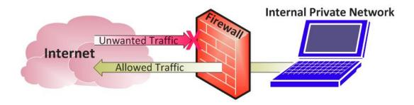
The firewall also provides protection between two networks, that is, it protects the protected network from an open external network. The advantages of the protection tool listed below, especially the packet filtering function, are an effective means of protection against DOS attacks. Package filters control:
