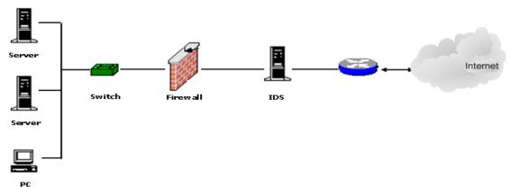
This system is divided into two main classes. It is divided into the Network Intrusion Detection System and the Host Intrusion Detection System. The principle of operation of the system of unauthorized access to the network (NIDS) is as follows:
