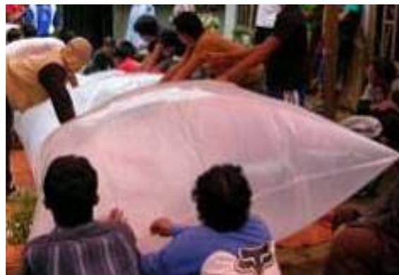
Figure 6. Leak test for digester.
