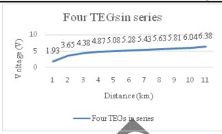
Figure 7 Graph of performance of four TEGs in actual setup
