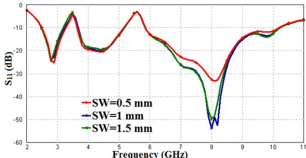
Fig.6 Effect of SW on Return Loss
