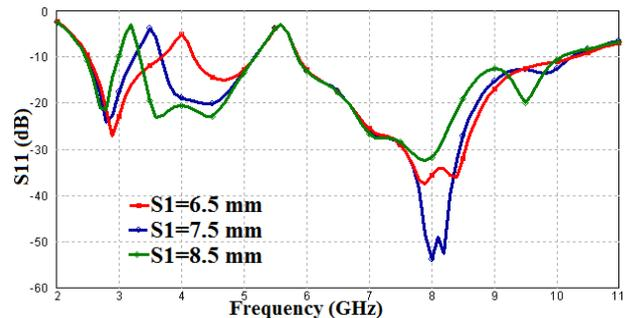
Fig.5. Effect of  $S_1$  on Return Loss
