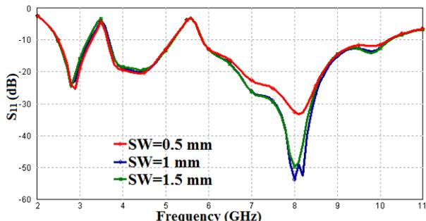
Fig.6 Effect of SW on Return Loss
