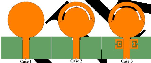
Fig.2 Antenna geometry: Case 1) simple UWB antenna, Case 2) UWB with Wi-Max band notch resonator, Case 3) UWB with WLAN band notch resonator
