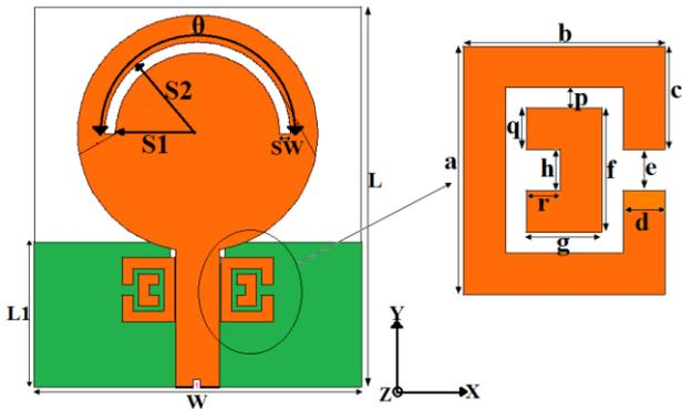
Fig.1. Geometry of antenna structure.
