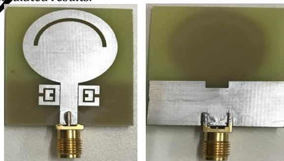
Fig.10 Fabricated structure
