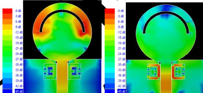
Fig.9 Surface Current distribution at, (a) 3.5 GHz, (b) 5.5 GHz
