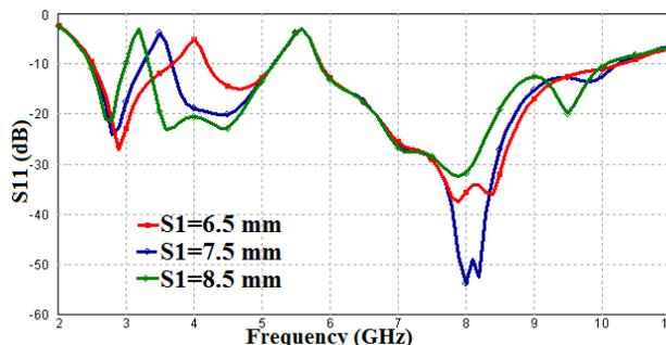
Fig.5. Effect of  $S_1$  on Return Loss
