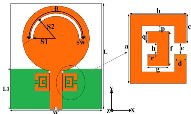
Fig.1. Geometry of antenna structure.
