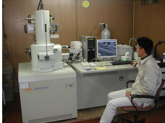
**Gambar 8.** Alat *Field Emission Scanning Electron Microscope* (FE SEM)
