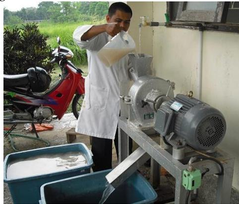
**Gambar 6.** Alat *disc refiner*
