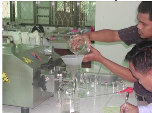
**Gambar 7.** Alat *high pressure homogenizer*
