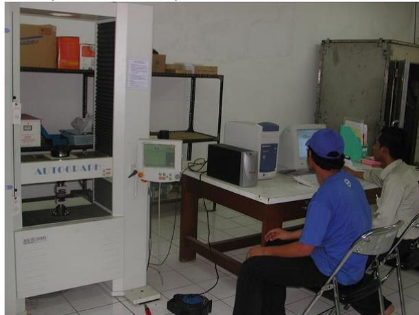
**Gambar 13.** Alat uji Universal Testing Machine (UTM)
