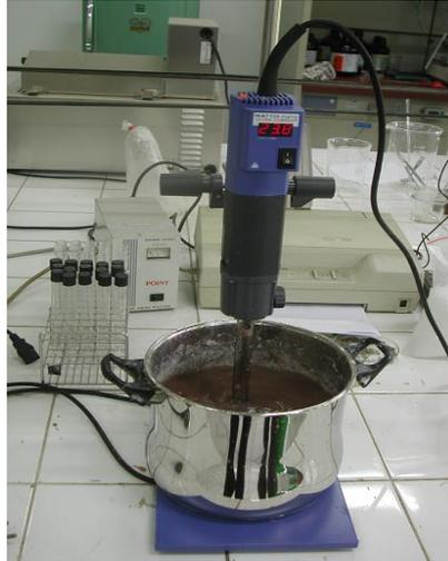
**Gambar 3.** Alat Ultra turrax T 25 (*dispersing machine*).
