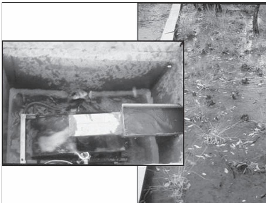
Figure 7. Collection of infiltration-excess, overland flow in one of the runoff troughs and associated tipping bucket during a storm.
