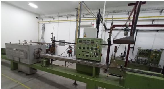
Figure 2. Heating furnace and quenching canal.
